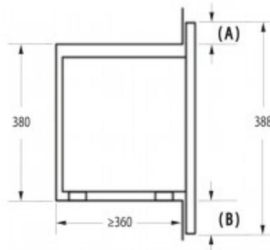
Installation of a microwave oven and frame overhangs:
